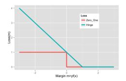
Hinge is a **convex**, **upper bound** on 0-1 loss. Not differentiable at m=1. We have a "margin error" when m<1.
